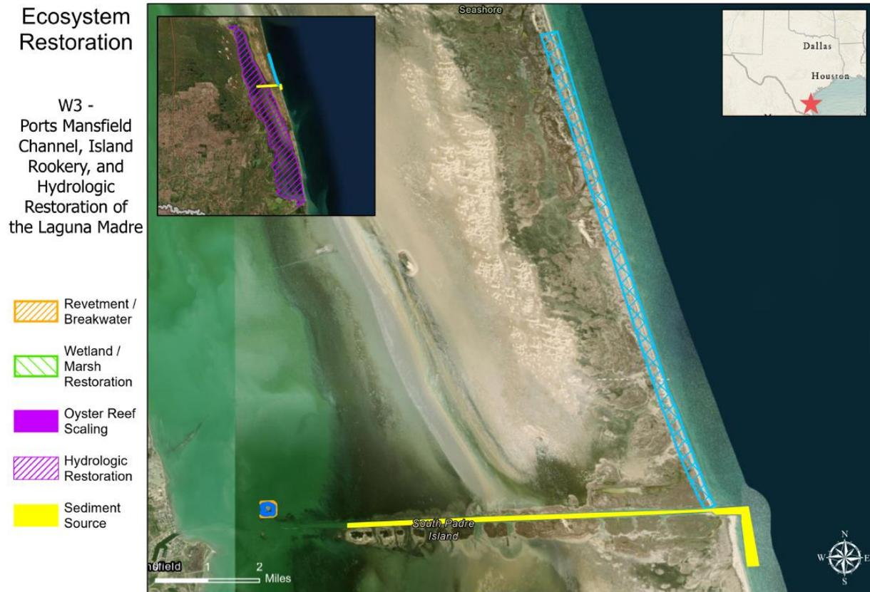
**Figure 2-20. ER Measure W-3: Port Mansfield Channel, Island Rookery, and Hydrologic Restoration**
